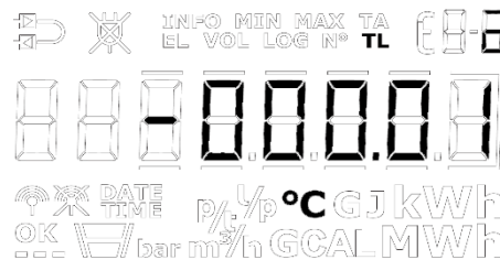
Figure 21 - Setting up negative TL2 in "SETUP loop", the - will be flashing when on the sign position and stays on when moving to another decimal.
