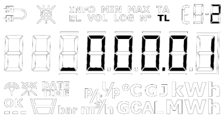
Figure 20 - Setting up positive TL2 in "SETUP loop", the _ will be flashing when on the sign position but disappears when moving to another decimal.
