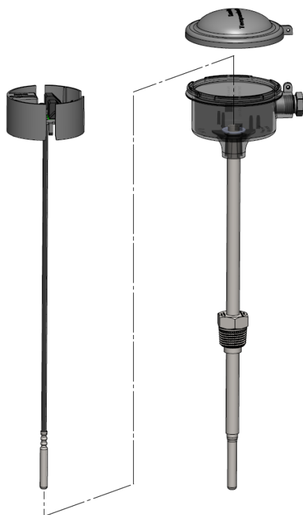
Figure 15: The \varnothing 5.8 mm pocket sensor with connection head can, for example, be mounted in a tee as shown in Figure 16.
