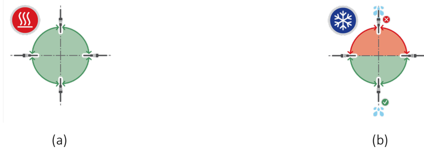
Figure 6. Acceptable orientation of a temperature sensor in (a) a heating and (b) a cooling application.
