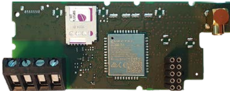
SIM card mounted in the module
