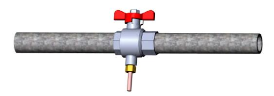
The ball valve is as far as possible installed as shown in the illustration. In case of cooling measurement, the ball valve should always be installed as shown by which you limit any problems with penetration of condensation in the temperature sensor. Installation of the temperature sensor in a ball valve ensures an optimal position in the liquid flow and thus contributes to a correct measurement of energy.
